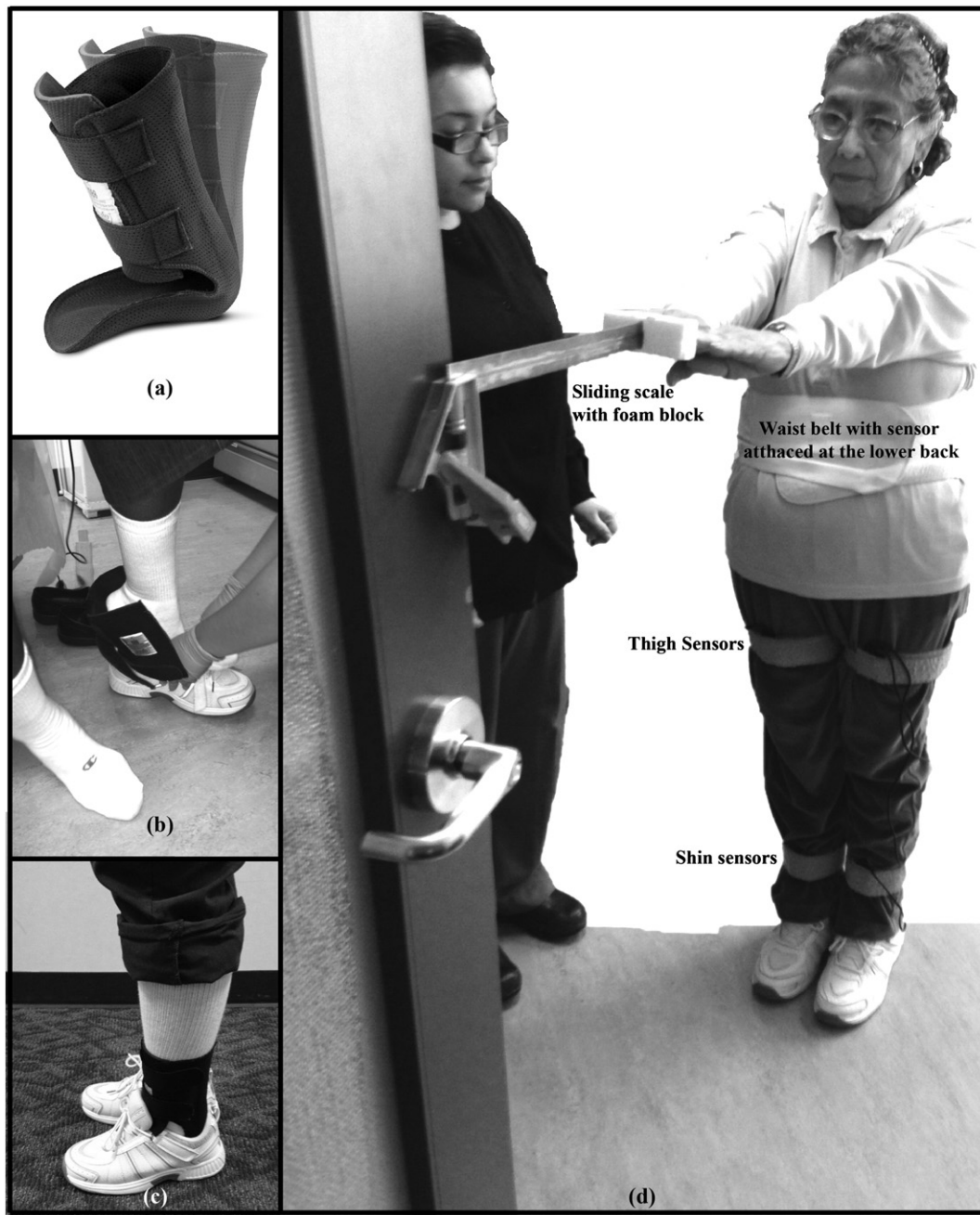
Fig. 1. (a) Open posterior leaf gauntlet style custom-made AFO (b) Participants sliding in their feet into the standard shoes (c) AFO placed inside the standard shoes (d) Functional reach task with sliding scale arrangement and body worn inertial sensors attached to the shin, thigh and the lower back.
